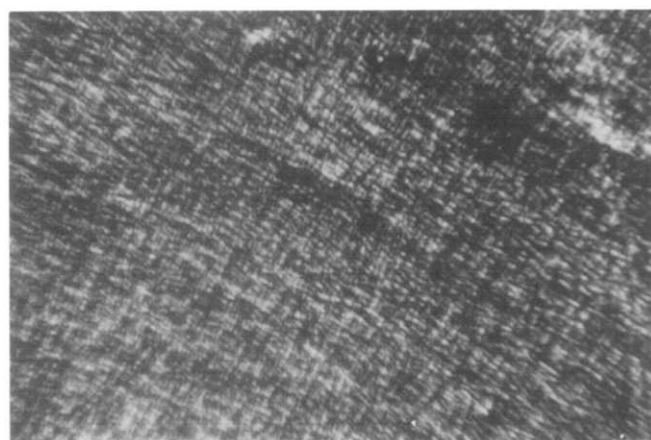
Figure 4 Morphology of crystalline PVK sample as seen under optical microscope (x320)
